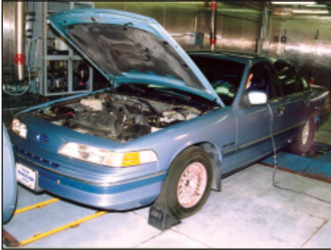
*Chassis Dynamometer Testing*
